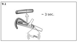
**9.1** Under start-up, keep pressing the Answer/End button for three seconds. Alternatively, remove the snap-on cover and press the reset button on the headset for three seconds.
